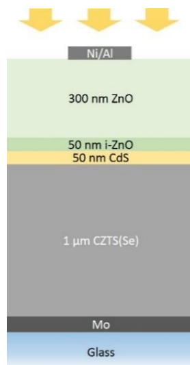
Figure 1.1. Cross-section of a typical CZTS(Se) solar cell device. This substrate configuration is illuminated on the front side of the diode. Charge carriers are generated and separated within the CZTS absorber layer. Holes are collected at the back contact (Mo), and electrons are collected at the front contact (Ni/Al). Cross-section of a typical CZTS(Se) solar cell device showing all layers that comprise a full device.
